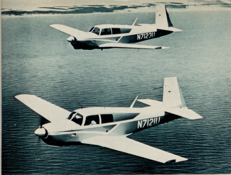
Mooney's Mark 21's: At the top is a standard Mark 21, the model Author Karant writes about in this article. The lower plane is the Super 21, which is powered by 200 h.p. fuel-injected Lycoming engine, and has a maximum cruise speed of 187 m.p.h. and a service ceiling of 19,500 feet
